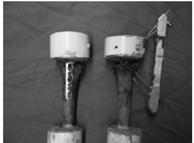
Fig. 1. Cadaveric distal radius fracture model in which the fractures were treated with either a CPX nonspanning external fixator (right) or a volar locking plate (left).
